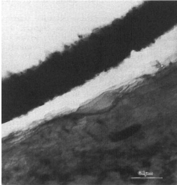
FIGURE 4 TEM micrograph of section through a fracture surface close to an aluminium surface etched prior to bonding.
